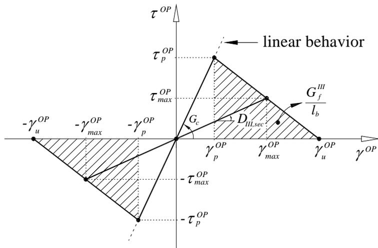
Fig. 3 -- Generic out-of-plane (OP) shear stress-strain diagram.
