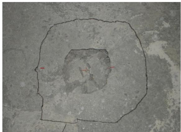
Figure 10. Punching critical contour.
